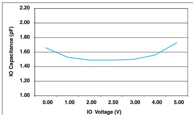
Figure 1. IO Capacitance vs IO Voltage (V<sub>CC</sub> = 5 V)
