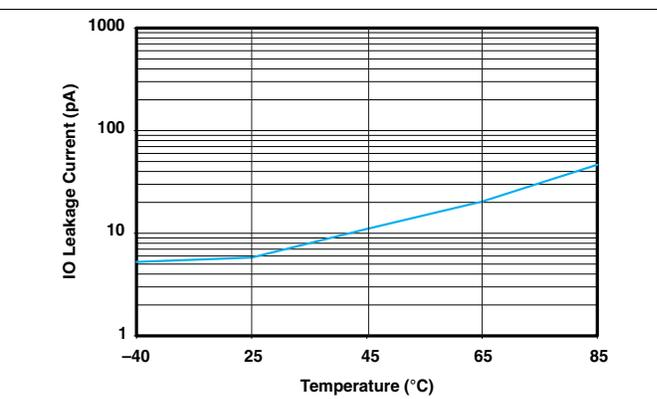
Figure 2. IO Leakage Current vs Temperature (V<sub>CC</sub> = 5 V)
