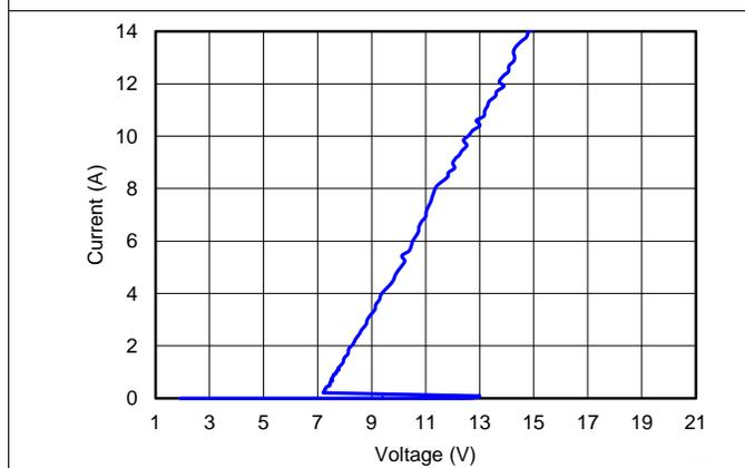
Figure 3. TLP IO to GND (DRS Package)
